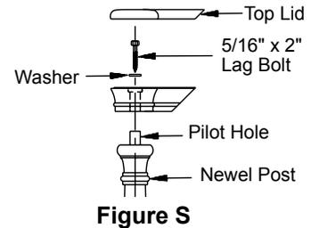
**Step 15 - Fasten Fitting to Post to Post Newel. (Figure T)**
